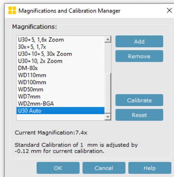
Note working distance of the current camera setup defined as the distance between the camera and the focused object shall not be changed after making the calibration. Altering working distance will change the magnification resulting in incorrect calibration.
