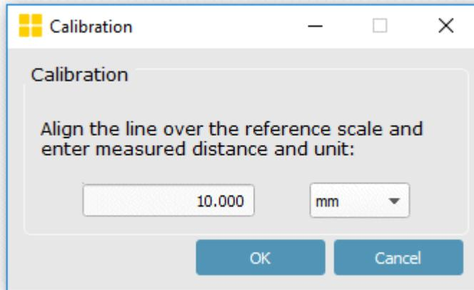
Select, drag, and align both ends of the calibration line to the matching lines on the reference image. Type in the distance and select the unit (**mm** or **µm**) in the calibration window. If imperial units are selected in Preferences, imperial units (**inch**, **mil**) will be shown in calibration window. Click OK to end the calibration process.
