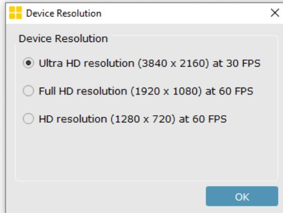
When attached to USB3.0 digital camera (BGA inspection system), Resolution and Format (aspect ratio) of the live image can be set according to the below tab. Default resolution for USB3.0 digital camera head is 2000x1500 pixels.
