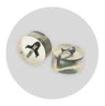
Glass window of the Inverted Microscope is simply replaced by any of the aperture window plates depending to size of the sample.
