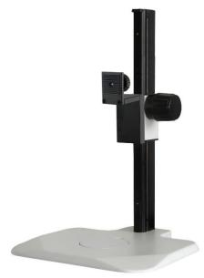
Provides flexibility for fine focusing of the image or working distance adjustment of Inspectis Digital Microscopes when used with different close-up lenses.
