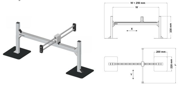
Custom cut linear guiding system mounted on high density aluminum profile for X-travel and a rigid custom sized double-arm boom creates requested Y-travel range of the Digital Microscope. The height of the linear guide can be adjusted and set to give the correct working distance of the Digital Microscope using 4x angle brackets. 4-direction tilt unit, Rack-&-Pinion Focusing module and Zmovement bracket are available for XY-travel Stand as extra accessories.
