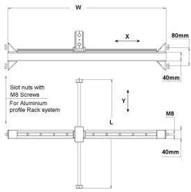
Custom cut linear guiding system mounted on high density aluminium profile for X-travel and a rigid custom sized double-arm boom for Y-travel. The X profile is fitted with mounting brackets to allow the correct setting of working distance during installation in the user's rack system. 4-direction tilt unit, Zextender bracket and camera grip handle are available for XY-travel Stand as extra accessories.
