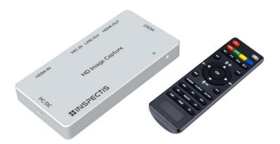
Compatible with HD (720p), Full HD (1080p) and 4K (2160p) output signals of Inspectis Digital Microscopes. Captures live video and still pictures up to 1080P resolution (1920x1080 pixels) via USB flash drive interface without need of host computer.
