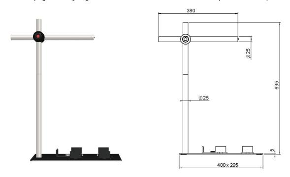
Provides complete flexibility for horizontal and vertical adjustment of Inspectis Digital Microscope. ESD-protected. Delivered with 5 pcs PCB holders and 4 pcs stainless steel pegs.
