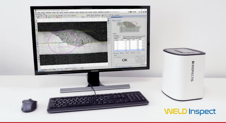
All-in-one Digital Inverted Microscope for weld bead analysis and measurement. Ultra HD imaging system with motorised zoom optics, auto-focus, built-in illumination, and dedicated software for weld measurements, documentation and reporting.
