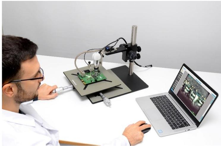
user to image from the first to up to 20 rows of BGA solder bumps with its flexible, electronically dimmable high-power LED fiber brush light as background illumination. The unique soft-touch mechanism design of the stand bracket protects the micro-prisms in the optical probe tip from damage when positioned on the surface of the PCB under inspection.
