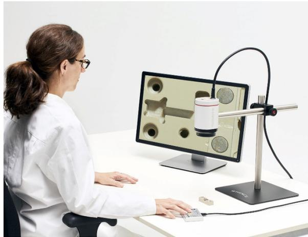
The U30 features fast responsive auto focus, he adds, making hand held inspection remarkably easy, allowing, an operator to quickly see, for example, if 01005 components are set properly.
